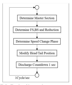
Fig.2. Flow chart of timer procedure.
